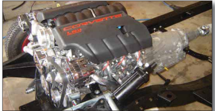
A close-up of the LS3 crate engine installed in the black 1957 Chevrolet Nomad.
